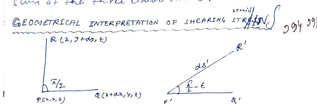
Consider three points P, Q, R in the undeformed state of the material such that the co-ordinates of P, Q and R are respectively  $(x, y, z)$ ,  $(x+dx, y, z)$ ,  $(x, y+dy, z)$ . The length of  $PQ = dx$  and that of  $PR = dy$  and the angle between  $PQ$  and  $PR$  is  $\frac{\pi}{2}$ .
