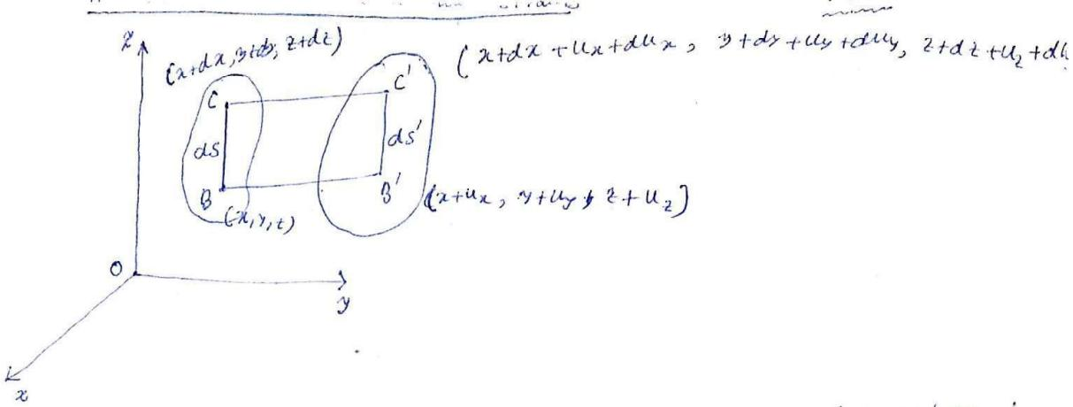
Let B and C be two infinitesimally close neighbouring points in a body before deformation and B' and C' are their new positions after deformation. The cartesian co-ordinates of these four points are as follows -
